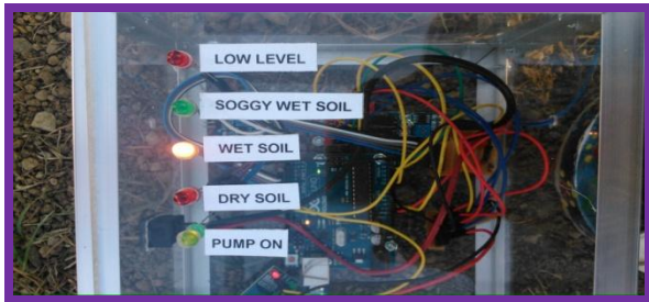
Figure 3.5.2 The soil condition is wet
