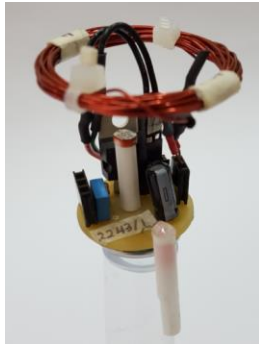
Fig. 6. Sample receiver module with coverings removed.
