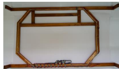
Fig. 3. Wooden canopy with LED strips and Transmitter Coils mounted.
