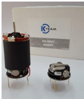
Fig. 7. KILOBOT with receiver module attached compared to original KILOBOT.
